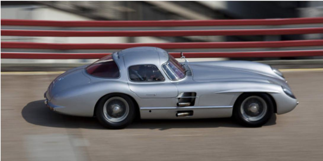
1955 Mercedes-Benz 300SLR 'Uhlenhaut' coupe an example of Mercedes-Benz' road/racing synergy. Fearsome and noisy coupe featured 3.0 liter straight 8 and 302 hp.
