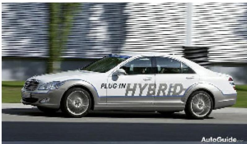
Already launched are the S400 Hybrid and the ML450 Hybrid. The S400 Hybrid was the first Mercedes hybrid to go on sale and is also the first mass production automobile to use a lithium-ion battery. Priced at \$87,950 it uses an electric motor and 3.5-liter gasoline V6 to produce 295-hp, while getting mileage of 19/26 mpg – an improvement of 26 percent over the S550 in the city. Despite its high-tech battery pack, the S400 Hybrid is a mild-hybrid, which limits its fuel economy.
